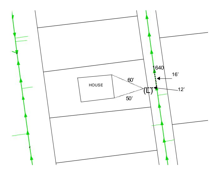
The (L) marks the location of the 2' high stake at the exact location that the owner would like the lateral stationed. The BTMA will terminate the 6" service lateral as close to the requested location as possible. When placing the stake at the location be sure that the stake poses no safety hazard and is not placed within a public right-of-way. All terminations must end a minimum of 1' beyond the owner's property line.
